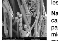
Nanovia AntiVirus SMNF 57 Membrane is designed to capture microorganisms (bacteria and viruses) and particulate matter in the air with a size less than 1 micron. The material belongs to the category of filter materials with filtration efficiency of PM 1.0 (ability to filter out viruses, bacteria and very fine dust particles.
