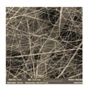
Nanovia AntiMicrobe products are laminated fabric that prevent penetration of microorganisms based on a mechanical collecting principle. Pore size in nanofibers structure are significantly smaller than the size of bacteria.
