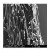
Innovative textile material that prevents penetration of dust mites and their allergens through the material based on mechanical collecting principle.
