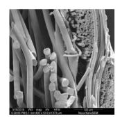
Anti permeability of Nanovia AntiAllergy fabrics for dust mites, alergens and bed bugs is ensured by nanofibrous layer which is closed inside the textile membrane.
